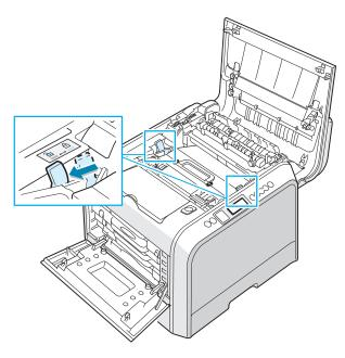
**5** Using the handle, lift the transfer belt out of the printer by lightly pulling it towards the left of the printer. Set it on a clean flat surface.
